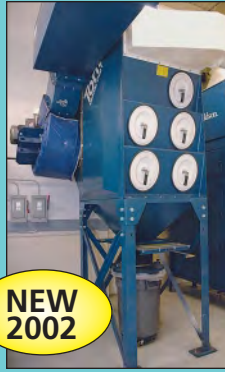
20 HP Torit Model DFO 3-10 Downflo Oval 1 Cartridge Type Dust Collector
