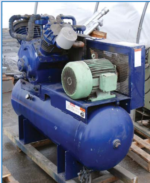
BRUNNER ENG & MFG 15 HP 200 GALLON 575 V 3 PHASE COMPRESSOR, MODEL A20301, 1755 RPM, TYPE W57V
