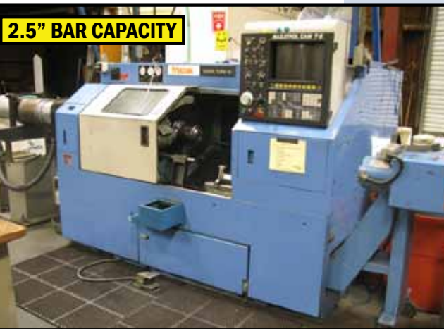
MAZAK QUICK TURN-15 CNC LATHE W/ MEZATROL T-2 CONTROL 10" CHUCK, S26 COLLET NOSE, 2.5" THROUGH HOLE.
