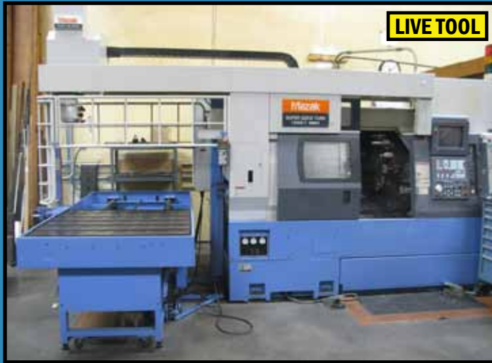
1998 MAZAK 15MS-Y MARK II CNC TURNING CENTER, W/ MEZATROL T-PLUS CONTROL, LIVE TOOL, FULL C-AXIS, 8" CHUCK, 6" SUB SPINDLE AND GL-100 GANTRY ROBOT
