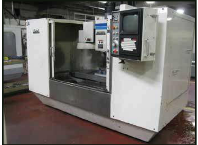
1993 VMC 4020 CNC VMC, 40 x 20 x 20 (XYZ), 40 TAPER, 10 HP MOTOR
