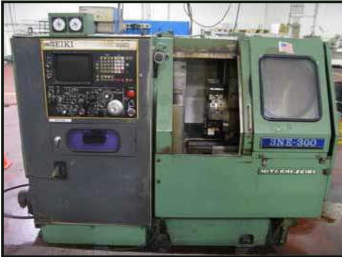
HITACHI SEIKI 3NE-300 CNC LATHE, 6" CHUCK W/ FANUC CONTROL
