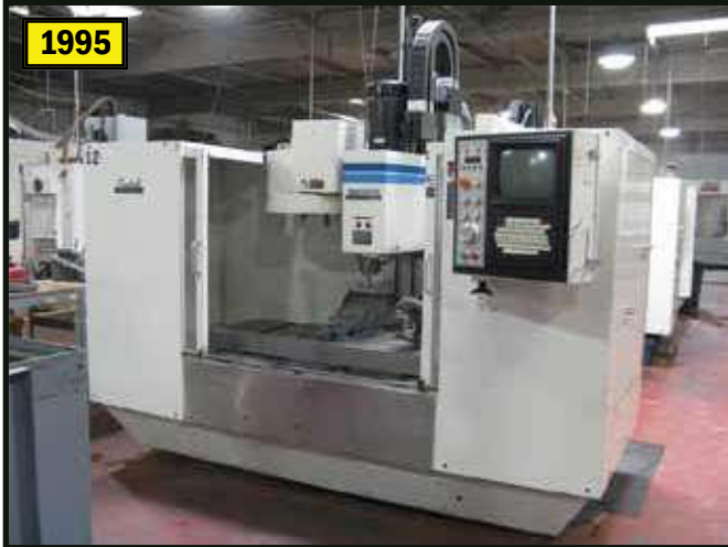
1995 FADAL VMC 4020 CNC VMC, 40 x 20 x 20 (XYZ)
