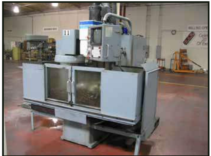
1986 VMC-40-904-1, CNC VMC, 22 x 16 x 20 (XYZ), 40 TAPER
