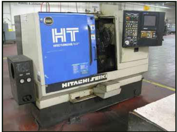
1993 HITACHI SEIKI HI-TECH TURN 20S11 CNC LATHE, 8" CHUCK W/ SEICOS L111 CONTROL
