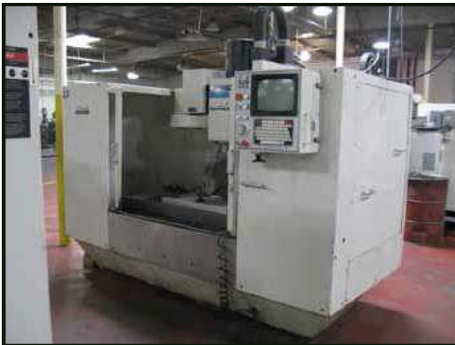
FADAL VMC 4020 CNC VMC, 40 x 20 x 20 (XYZ), 40 TAPER, 10 HP MOTOR
