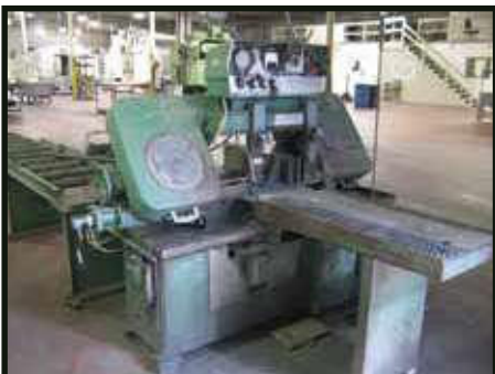
DO ALL C-70 HORIZONTAL BAND SAW, 12" x 12" CAP W/ FEED
