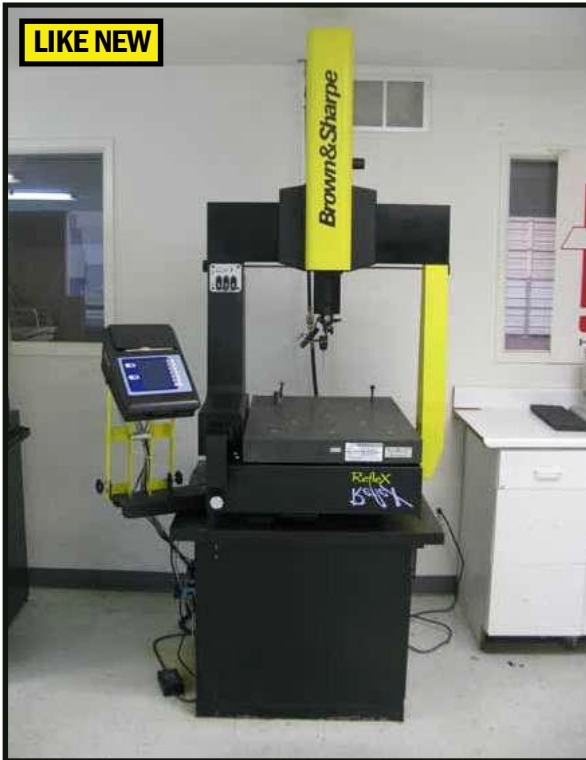
BROWN & SHARPE 3 AXIS CMM, 18" x 20" x 16" TRAVELS, MODEL REFLEX-454
