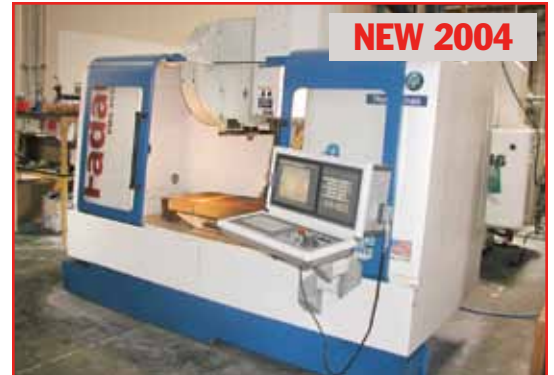
FADAL 4020 VMC, w/FANUC 18MBS 5-AXIS CONTROL
