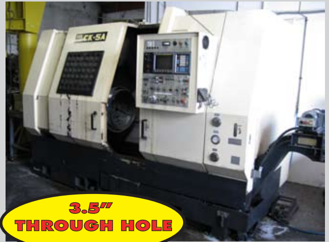
YAM CK-5A CNC LATHE, W/FANUC OT CONTROL, 15" CHUCK, 8 POSITION TURRET, 3.5 THROUGH HOLE
