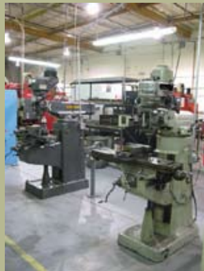
VIEW OF VERTICAL MILLING MACHINES
