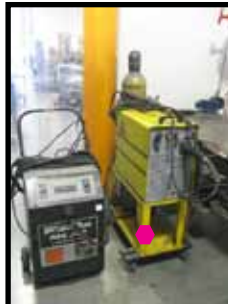
PARTIAL VIEW OF WELDERS AND PLASMA CUTTER
