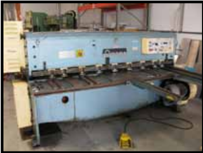
AMADA 8 FT x .25" MECHANICAL SHEAR MODEL M3060, W/ CNC BACK GAGE
